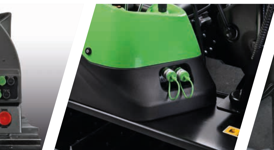
> 5 KF / 5 KM always offer 2 mid-mounted hydraulic connections.
