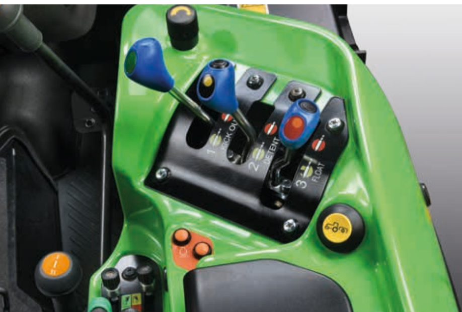
> Easy engagement of rear PTO via pushbutton.
