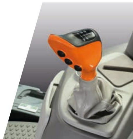
> Ergonomska prestavna ročica z gumbi ComfortClutch, APS in Powershift.
